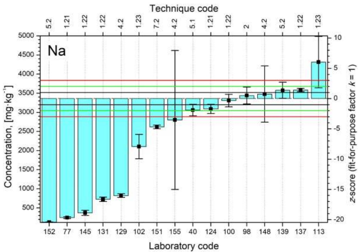
FIG. 40. Distributions of z-scores for analyte Na.
