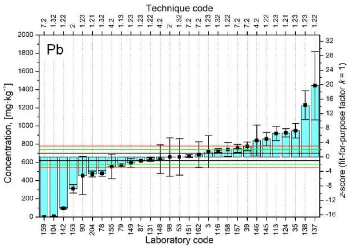
FIG. 43. Distributions of z-scores for analyte Pb.
