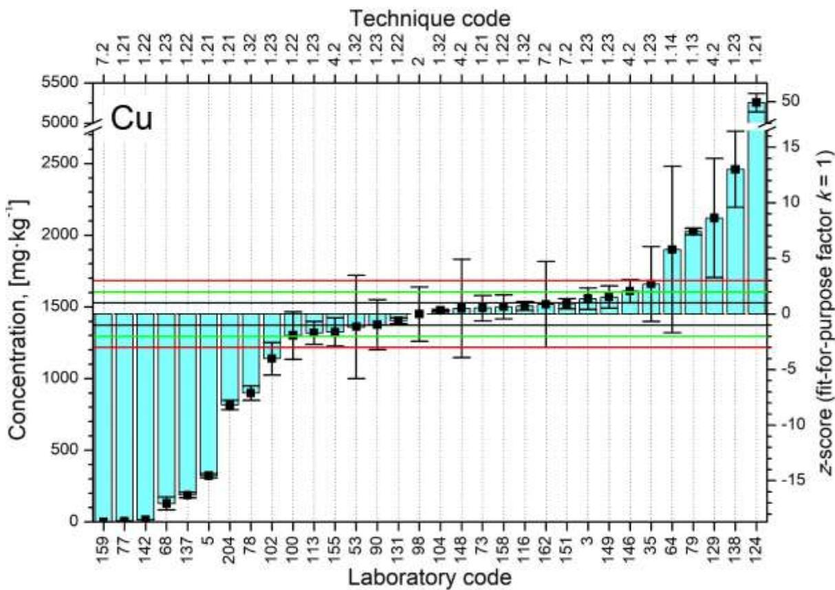
FIG. 34. Distributions of z-scores for analyte Cu.
