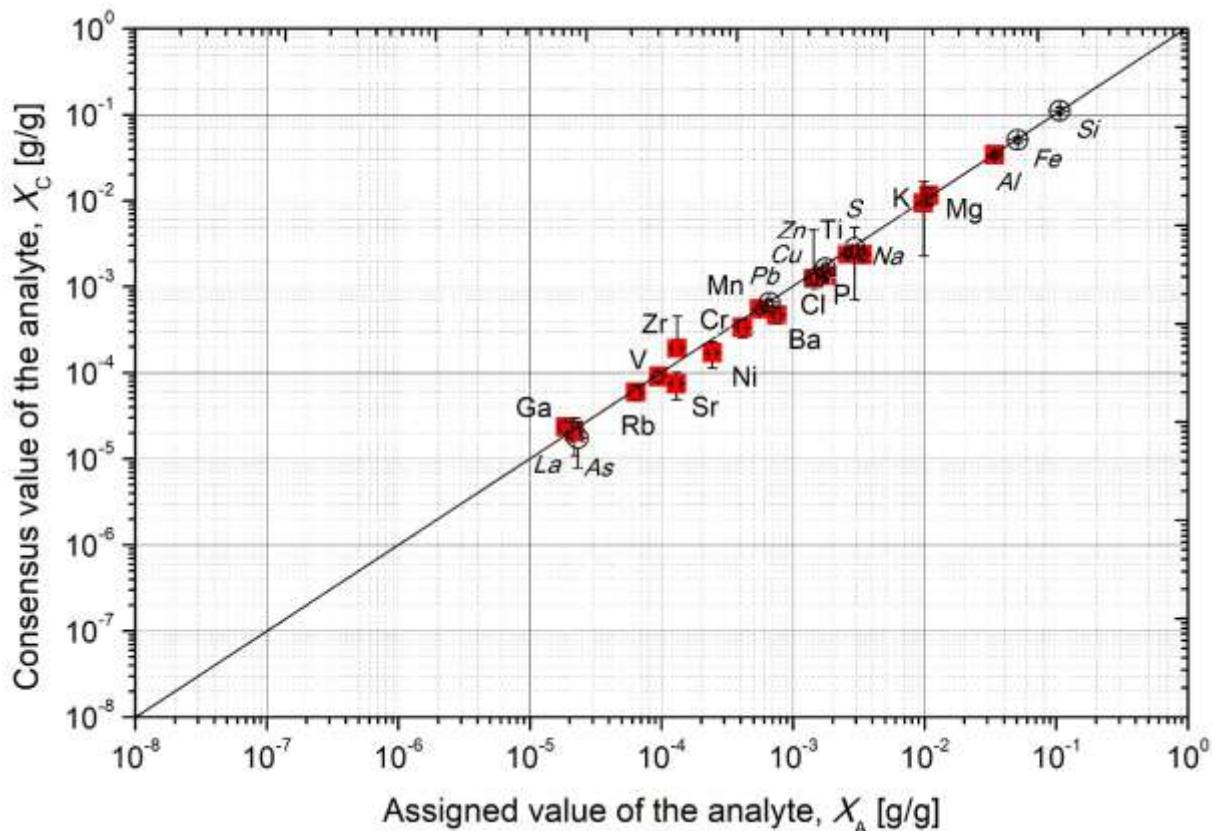
FIG. 2. Correlation between assigned,  $X_A$ , and consensus values of analytes,  $X_C$ <sup>1</sup>.
