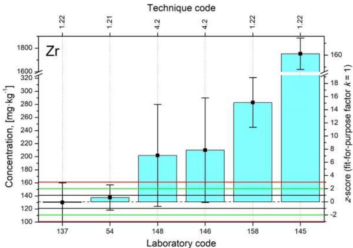
FIG. 51. Distributions of z-scores for analyte Zr.
