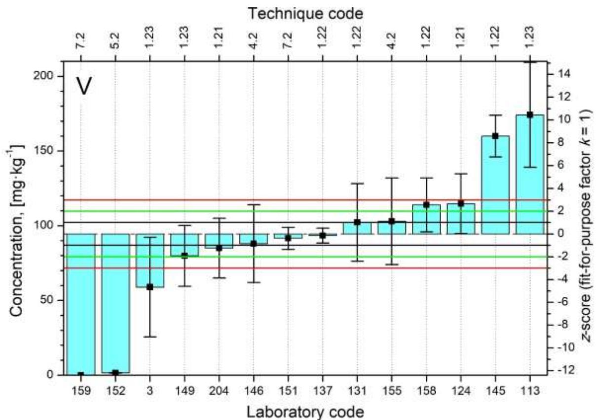
FIG. 49. Distributions of z-scores for analyte V.
