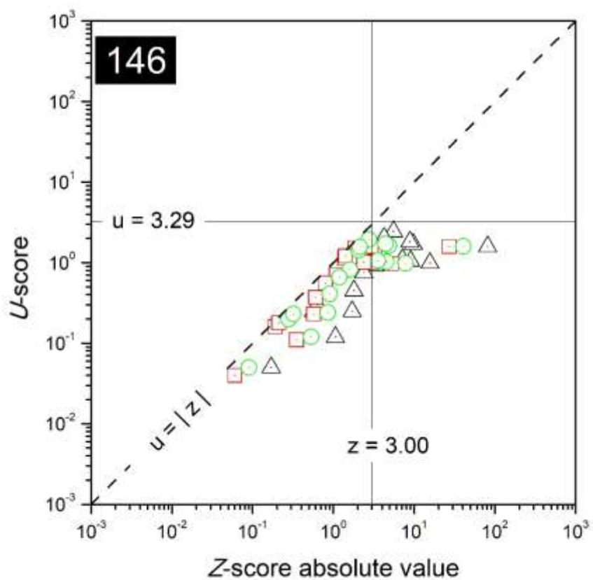
FIG. 83. Combined plots of  $z$ - and  $u$ -scores for the laboratory with code 146.
