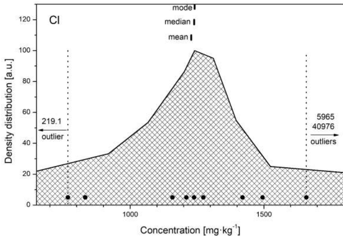
FIG. 7. The density distribution function for the analyte Cl.
