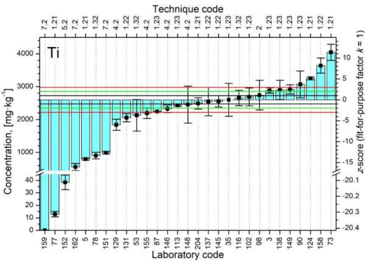
FIG. 48. Distributions of z-scores for analyte Ti.
