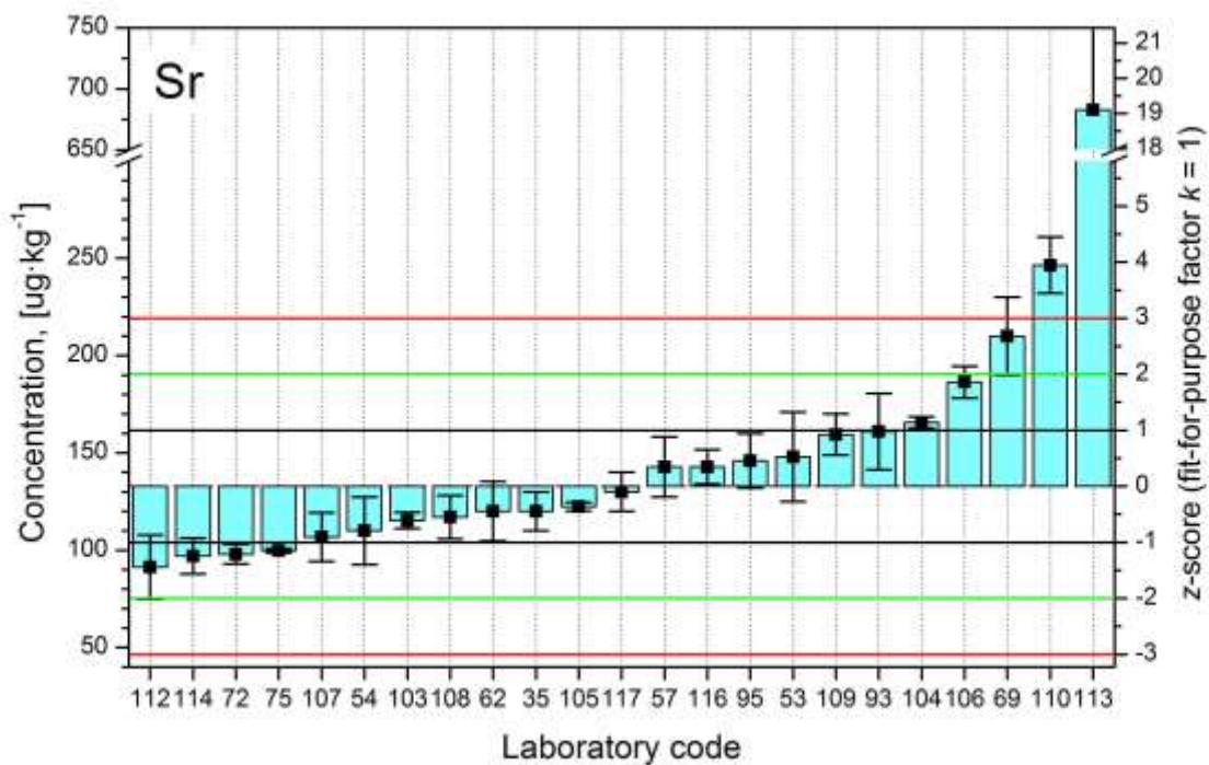
FIG. 88. Distributions of z-scores for analyte Sr in case of sample “3”.
