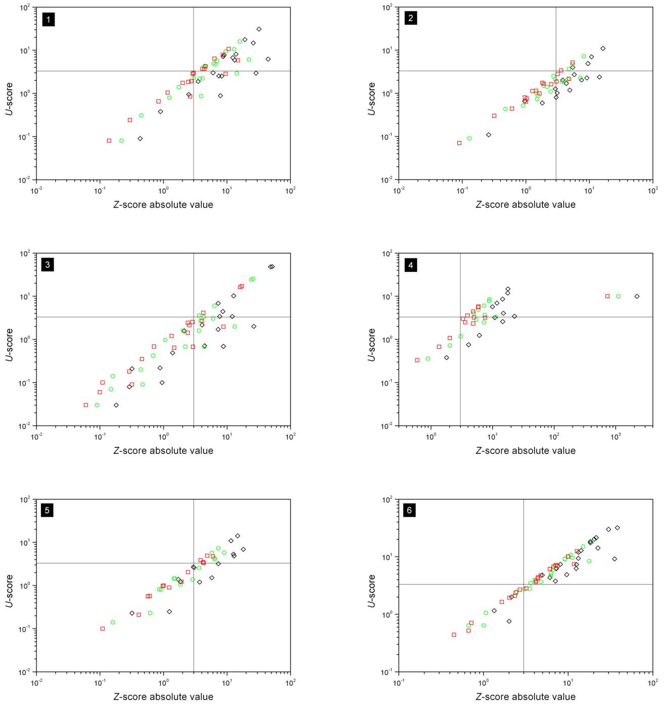
Fig. 5. Combined plots of  $z$ -scores and  $u$ -scores for participating laboratories. The laboratory code is shown in left upper corner of each plot. The hollow symbols denote the values calculated for specific fit-for-purpose levels as defined in Eqn. (2);  $k = 0.5$  (black diamond symbols),  $k = 1.0$  (green circle symbols), and  $k = 1.5$  (red square symbols). The solid lines mark the decision level for  $z$ -score,  $|z| = 3$ , and  $u$ -score,  $u = 3.29$ .
